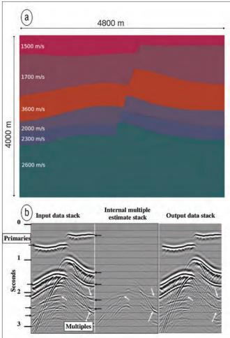
Figure 7. (a) A 2D synthetic model characterized by gently curved reflectors intersected by a fault. (b) The left panel shows a common-offset display from the synthetic data set created using the model. The middle panel shows the predicted internal multiples and the right panel is the result after subtracting the predicted multiples from the input data set. (From Matson et al., 1999, and Weglein et al., 2003)
