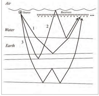
Figure 1. Marine primaries and multiples: 1, 2 and 3 are examples of primaries, free-surface multiples, and internal multiples, respectively.
