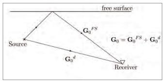
Figure 2. The marine configuration and reference Green's function.
