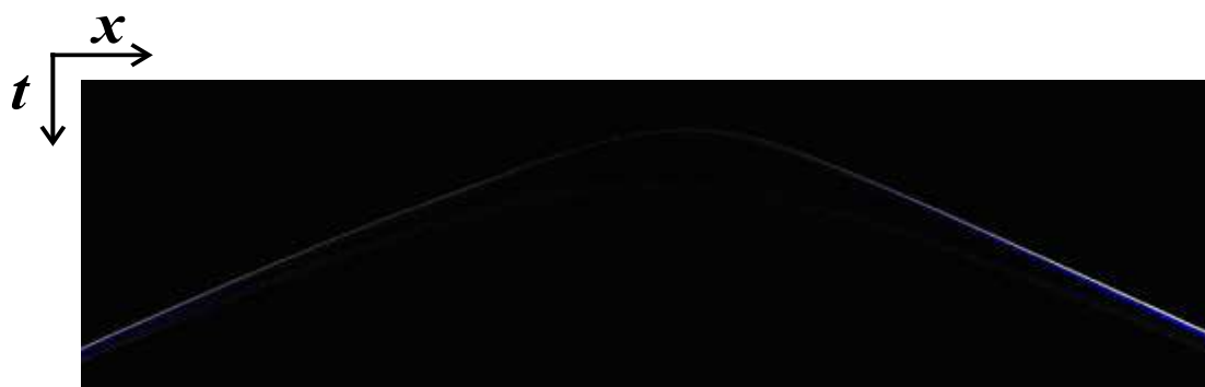
Figure 2: Typical shot gather computed using a finite difference numerical scheme. The source wavelet is the first derivative of a Gaussian.
