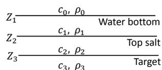
Figure 2: A 1D earth model, with three interfaces. The first interface, with depth  $Z_1$  is the water bottom. The second interface, with depth  $Z_2$ , can be identified with the top salt and the third interface, with depth  $Z_3$ , can be identified with the target.
