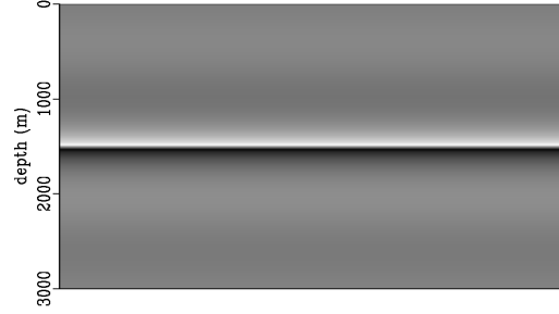
Fig. 10: The new M-OSRP Claerbout III (Stolt extended) migration for 2 way wave propagation. The example with c_0/c_1 velocity. The image both above and beneath the reflector. No "rabbit ears". Consistent image along the reflector. Light color image from above. Dark color image from below. (Qiang Fu and Weglein, 2015)
