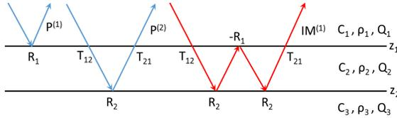
Figure 1: A two-reflector 1D model.  $P^{(1)}$  and  $P^{(2)}$  are primaries from the first and the second interface, respectively;  $IM^{(1)}$  is the first order internal multiple;  $R_1$  and  $R_2$  are reflection coefficients;  $T_{12}$  and  $T_{21}$  are transmission coefficients;  $c_1, c_2$  and  $c_3$  are the velocities;  $\rho_1, \rho_2$  and  $\rho_3$  are densities; and  $Q_1, Q_2$  and  $Q_3$  are quality factors.
