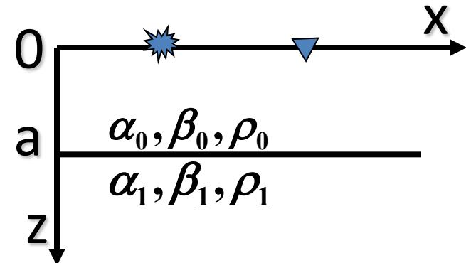
**Model 1: shale (0.2 porosity) over oil sand (0.1 porosity)**
