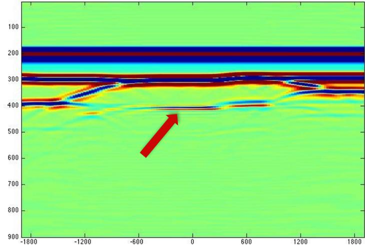
For the case of an interfering internal multiple and base salt primary, the ISS elimination removed the internal multiple without damaging the primaries (Yanglei Zou, Chao Ma, and A. Weglein, 2018)
