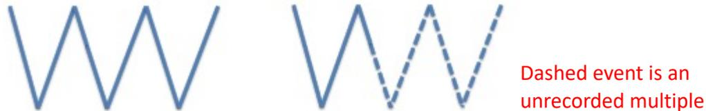
Using a recorded multiple to find an approximate image of an unrecorded primary of the multiple: illustrates the need to remove unrecorded multiples. A solid line (—) is a recorded event, and a dashed line (---) connotes an unrecorded event.
