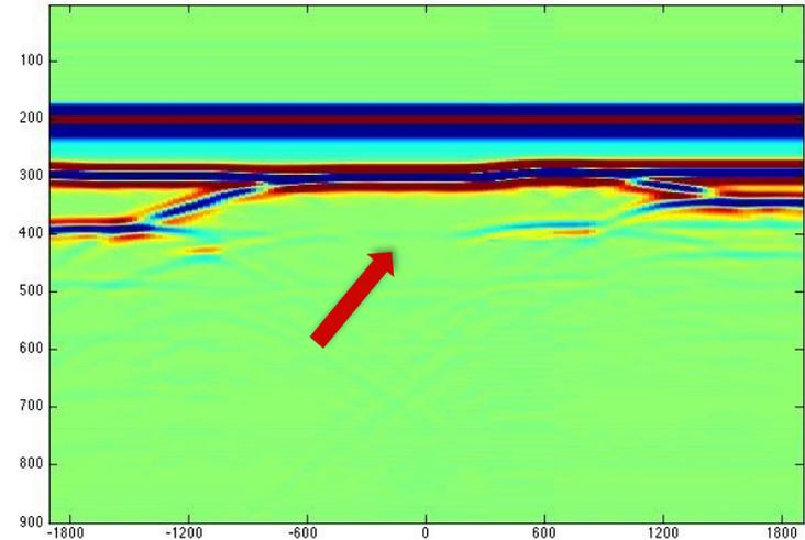
**For the case of an interfering internal multiple and base salt primary, the ISS internal multiple attenuation + adaptive damage the primaries (Yanglei Zou, Chao Ma and A. Weglein, 2018)**
