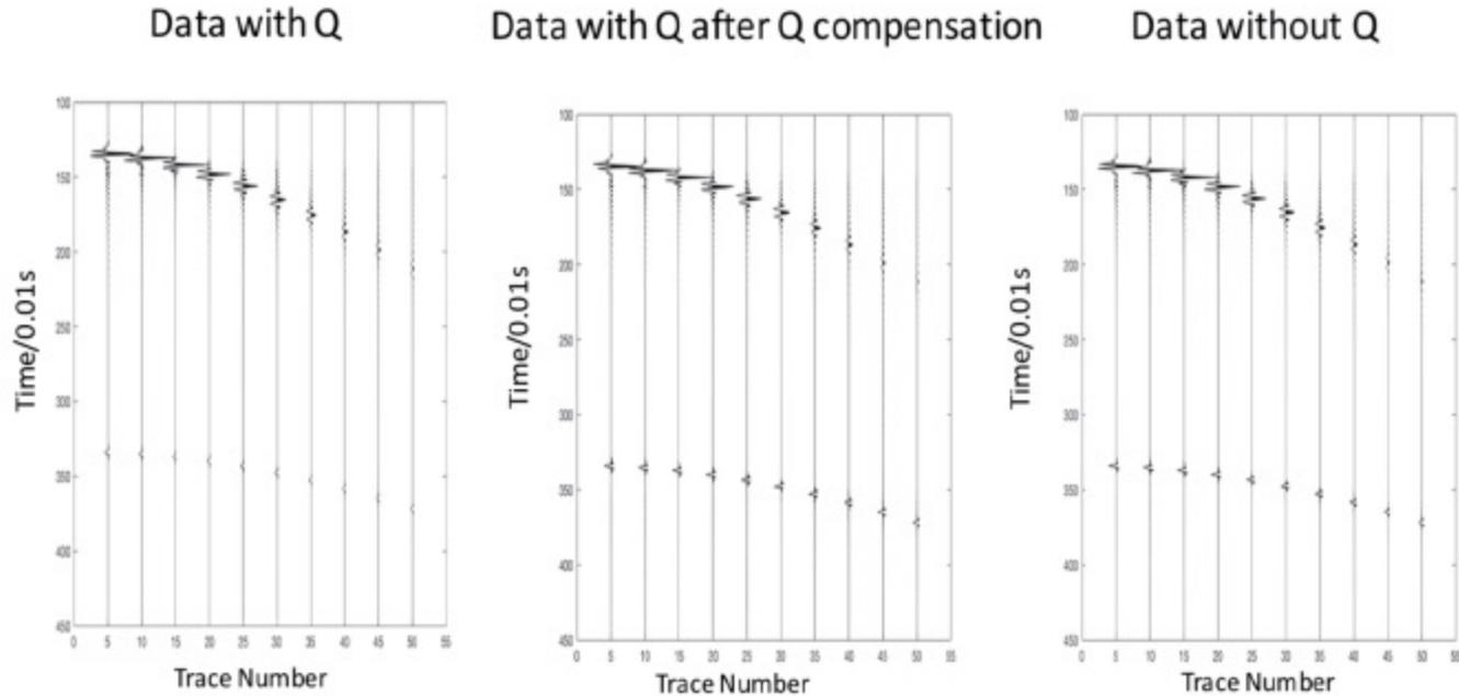
Fig. 2. Left: Data generated by the model with  $Q$ . Middle: The data (with  $Q$ ) after ISS  $Q$  compensation without knowing or estimating  $Q$ . Right: Data generated by the same model but without  $Q$ .
