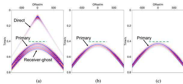
Figure 7: Deghosting results with a flat free surface and a flat cable. (a) the total pressure; (b) deghosted data at E.S.; (c) deghosted data at cable. Green lines locate the arrival time of data's primary.
