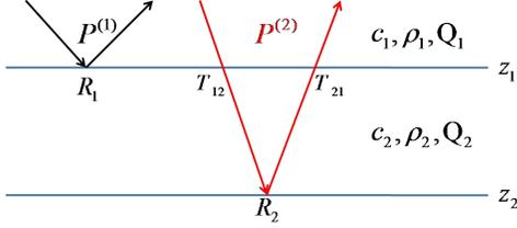
Figure 1: A two-reflector 1D model.  $P^{(1)}$  and  $P^{(2)}$  are primaries from the first and the second interface, respectively;  $R_1$  and  $R_2$  are reflection coefficients;  $T_{12}$  and  $T_{21}$  are transmission coefficients;  $c_1$  and  $c_2$  are the velocities;  $\rho_1$  and  $\rho_2$  are densities; and  $Q_1$  and  $Q_2$  are quality factors.
