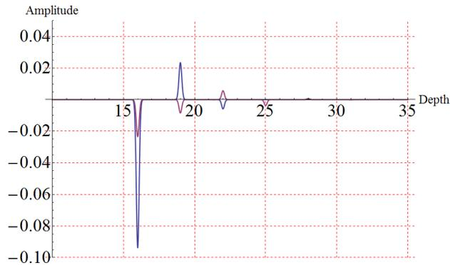
Figure 4: Comparison between  $D$  (**blue**) and  $D + D_3$  (**purple**). The comparison shows the contributions of  $D_3$  are (1) reducing the first-order internal multiples and (2) altering the amplitude of the higher-order internal multiples. Notice that, only internal multiples are plotted in  $D$ .
