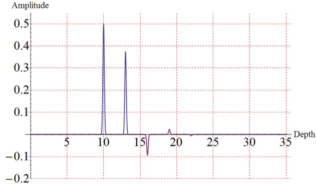
Figure 3: Input data in pseudo-depth domain. **Blue** and **purple** lines represent primaries and internal multiples, respectively. There are two primaries at depths 10 and 13 and three internal multiples at pseudo-depths 16 (first-order), 19 (second-order), and 22 (third-order).
