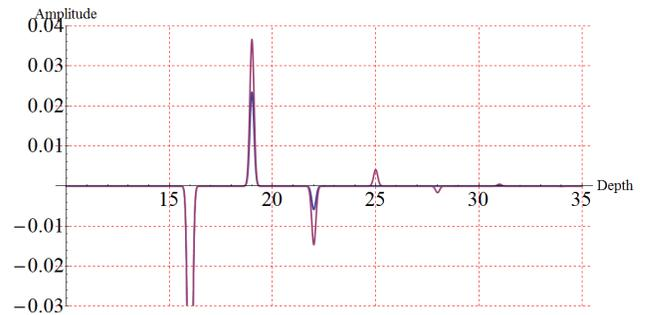
Figure 6: Comparison between  $D$  (blue) and  $D + D_5$  (purple). Without the contribution from  $D_3$ ,  $D + D_5$  will **increase** the amplitude of the second-order internal multiple. In other words, alteration of higher-order internal multiples by  $D_3$  is necessary for their attenuation.
