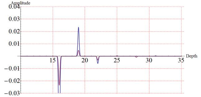
Figure 5: Comparison between  $D$  (blue) and  $D + D_3 + D_5$  (purple). Comparing Figure 4 and 5, it is concluded that adding  $D_5$  to  $D + D_3$  will further reduces second-order internal multiple.
