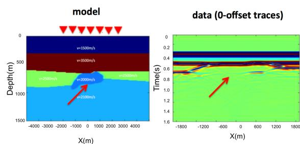
Figure 5: Zero offset traces of data. Note the interfering internal multiple and base salt primary.
