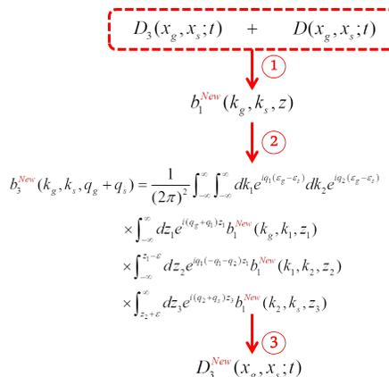
Figure 3b: In a 2D case, the workflow of the new ISS internal-multiple-attenuation algorithm with the addressing of the spurious events. The steps are same as in Figure 3a, but using a new input.  $D_3(x_g, x_s; t)$  is the output from the current algorithm in Figure 3a.
