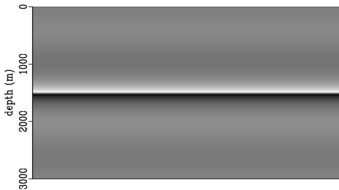
Figure 6: Zoom-in of Figure 4 The new M-OSRP Claerbout III (Stolt extended) migration for 2 way wave propagation. The example with c_0/c_1 velocity. The image both above and beneath the reflector. No “rabbit ears”. Consistent image along the reflector. Light color – image from above. Dark color – image from below. (Qiang Fu and Weglein, 2015)
